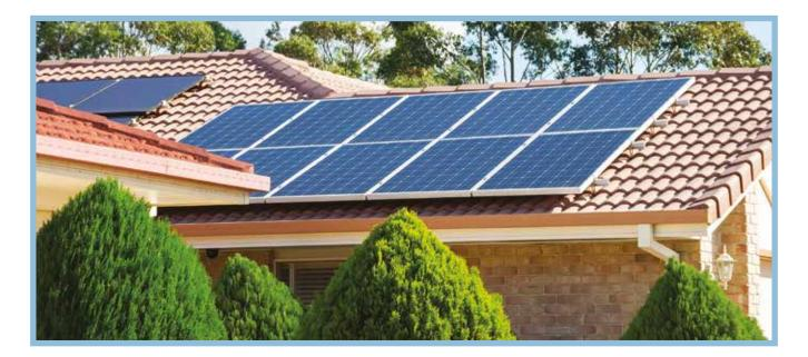
Before installing a solar PV system, you'll need to ensure the panels will be in a sunny area. They should also slope at an appropriate angle and face the right direction. Solar panels work best if installed facing north at 30 degrees from horizontal. If you install the panels with the wrong slope or direction it will reduce the amount of power generated.
